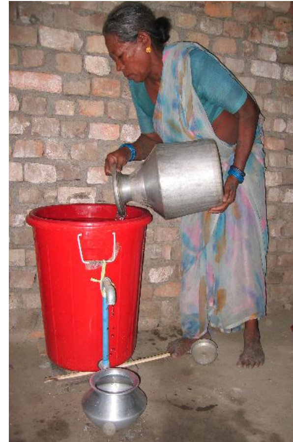
Kanchan Arsenic Filter
